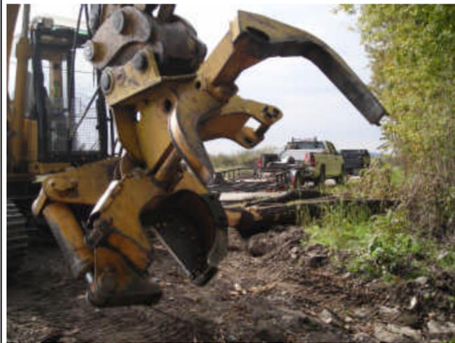
**Excavator-mounted tree shear**
